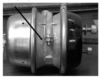
Insert the detachable release bolt through hole in head. Turn the release bolt clockwise until it stops and locks, then pull the release bolt out as far as possible, and run the nut down, holding the bolt in place.
